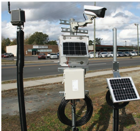
Low-cost flood gauges being tested in Lumberton.
