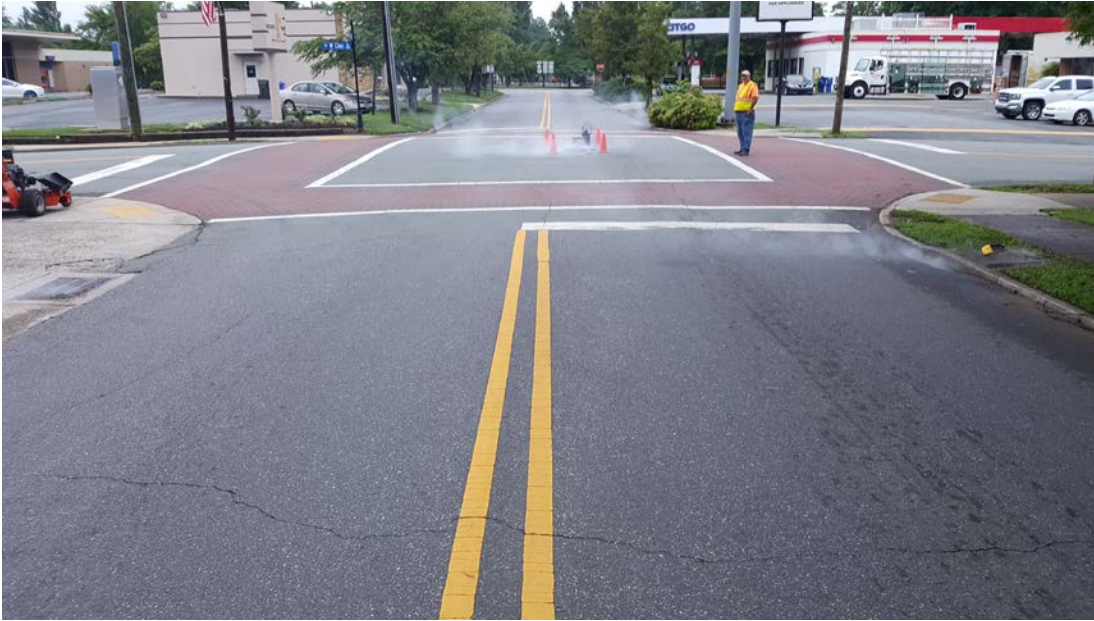
Figure 15: Typical Smoke from Storm Drainage via Sewer System Smoking
